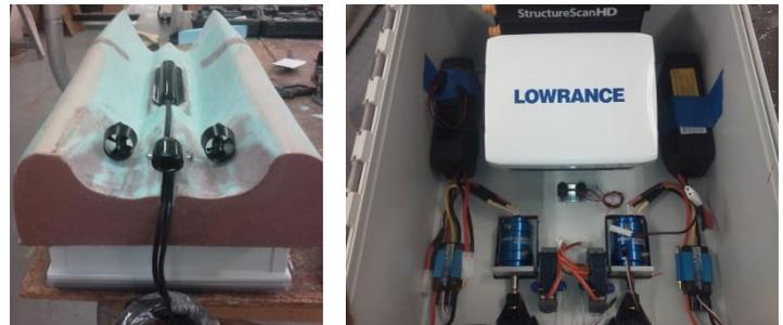
BathyBoat collects sonar data using a Lowrance HDS Sector Scan System. This allows for down looking (50 and 200 kHz) Side Scan Sonar with data recording and GPS in a single unit. This is combined with an internal GPS which collects a positions at 5Hz. This sonar allows for a high density of points to be collected as it can store up to 12,000 points internally. Bathyboat can be customized to use other sonar systems.
