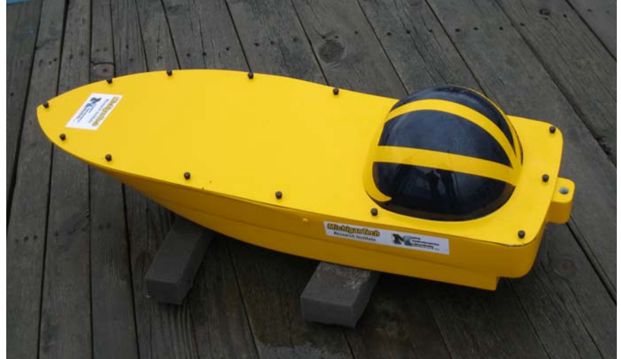
Figure 1. BathyBoat is three feet in length and weighs 30 pounds.
